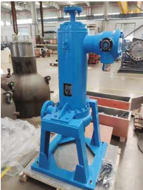
Vinyl Chloride Monomer Pump used in manufacturing of PVC.
