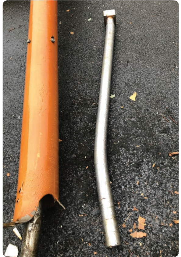
Bent drive shaft
