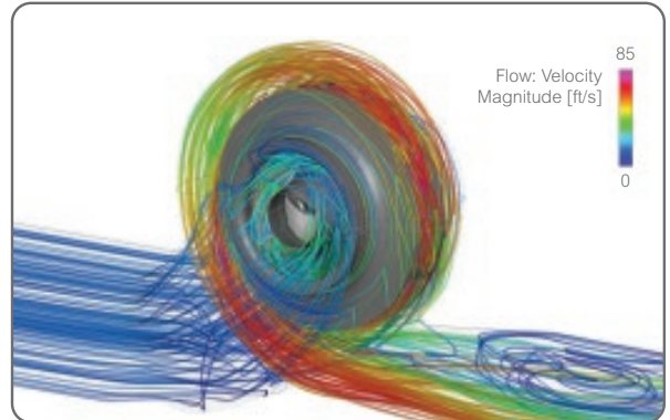
CFD model showing impeller and velocity streamlines
