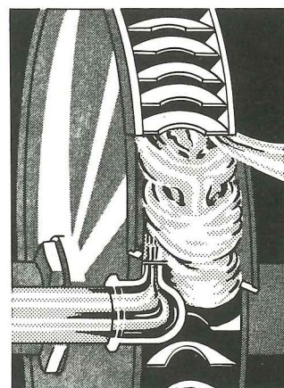
Path of steam from jet to wheel
