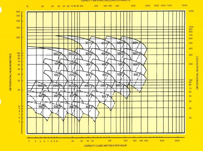
A full range of 50 cycle curves available. Capacities to 480m3/H. Heads to 220M.
